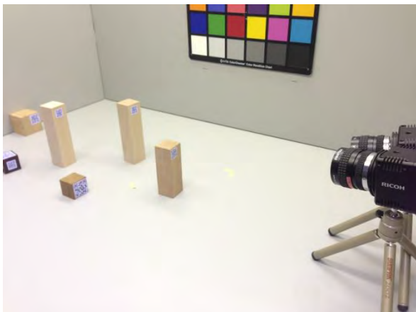
被写界深度拡大カメラ (EV-G030B1 & EL-CC0833B-VG)
